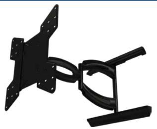
Articulating mount for 32" to 75" displays. Multiple joint arm holds display 3.5" from wall when retracted and 27" when fully extended. Smooth tilt adjustments of +15° (forward) and -5° (back) with a locking knob and 3° side-to-side roll facilitates a variety of viewing angles and perfect positioning. Integrated cable management for clean look.
