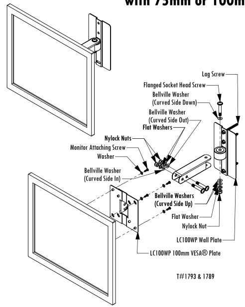
Wood Lag Screws are provided for wood stud installations. For concrete or metal sutds, use the WMAAB3, concrete anchor bolt kit, or WMATB3, toggler bolt kit, and follow the instructions specific to these fasteners.
